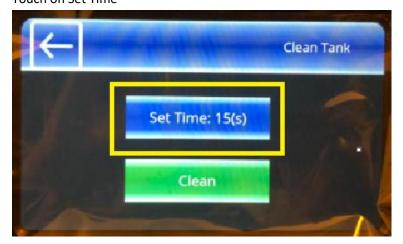
> Insert the Time in between 5 to 15 seconds to project the UV light on the platform & touch enter
